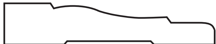
SM 444 1\frac{1}{16} x 3\frac{1}{4} - PINE, PRIMED \frac{9}{16} x 3\frac{1}{4} - RED OAK \frac{5}{8} x 3\frac{1}{4} - MDF
