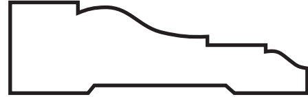
SM 366 1\frac{1}{16} x 2\frac{1}{4} - PINE, PRIMED \frac{9}{16} x 2\frac{1}{4} - RED OAK \frac{5}{8} x 2\frac{1}{4} - MDF
