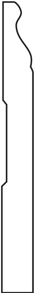
SM 163 (A & B AVAILABLE IN 1/2") A - \frac{9}{16} X 5\frac{1}{4} - MDF B - \frac{9}{16} X 7\frac{1}{4} - MDF C - \frac{11}{16} X 9\frac{1}{4} - MDF
