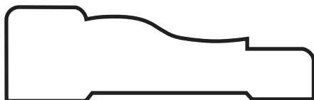
SM 356 1\frac{1}{16} x 2\frac{1}{4} - PINE, PRIMED \frac{9}{16} x 2\frac{1}{4} - RED OAK \frac{5}{8} x 2\frac{1}{4} - MDF
